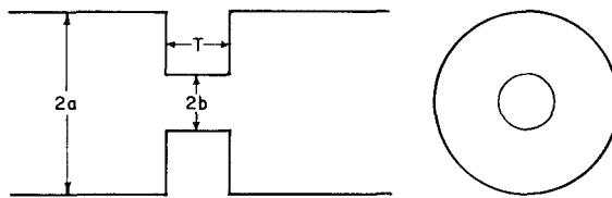
Fig. 1. Thick circular iris in circular waveguide.
